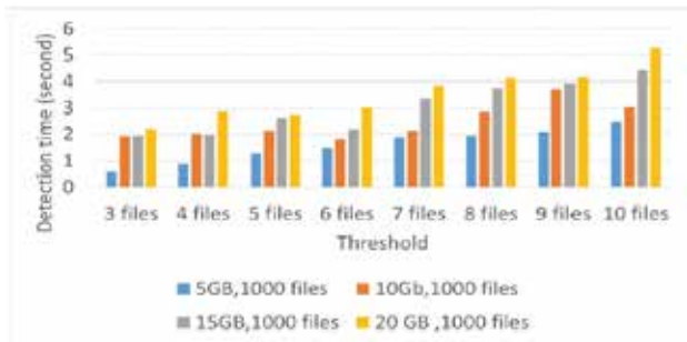
Fig. 2. Detection time vs the threshold for 1000 files-system of different sizes 5GB, 10GB, 15GB and 20GB [2]
