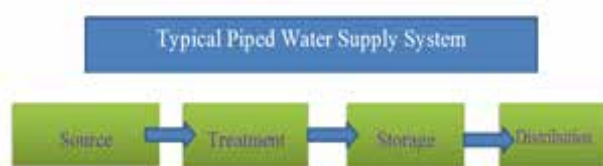
Fig.1: Process of water supply system
