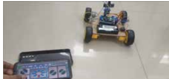
Fig 9: Shows the Bluetooth controller and the movement of the likewise robot in Left, Right, Forward and Backward direction
