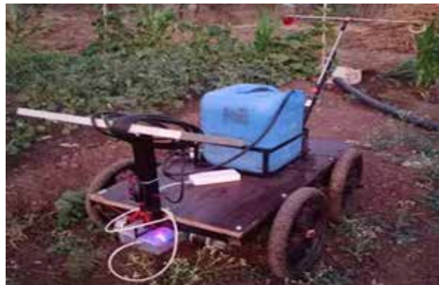
Fig 4: Developed Autonomous Pesticide Sprayer
